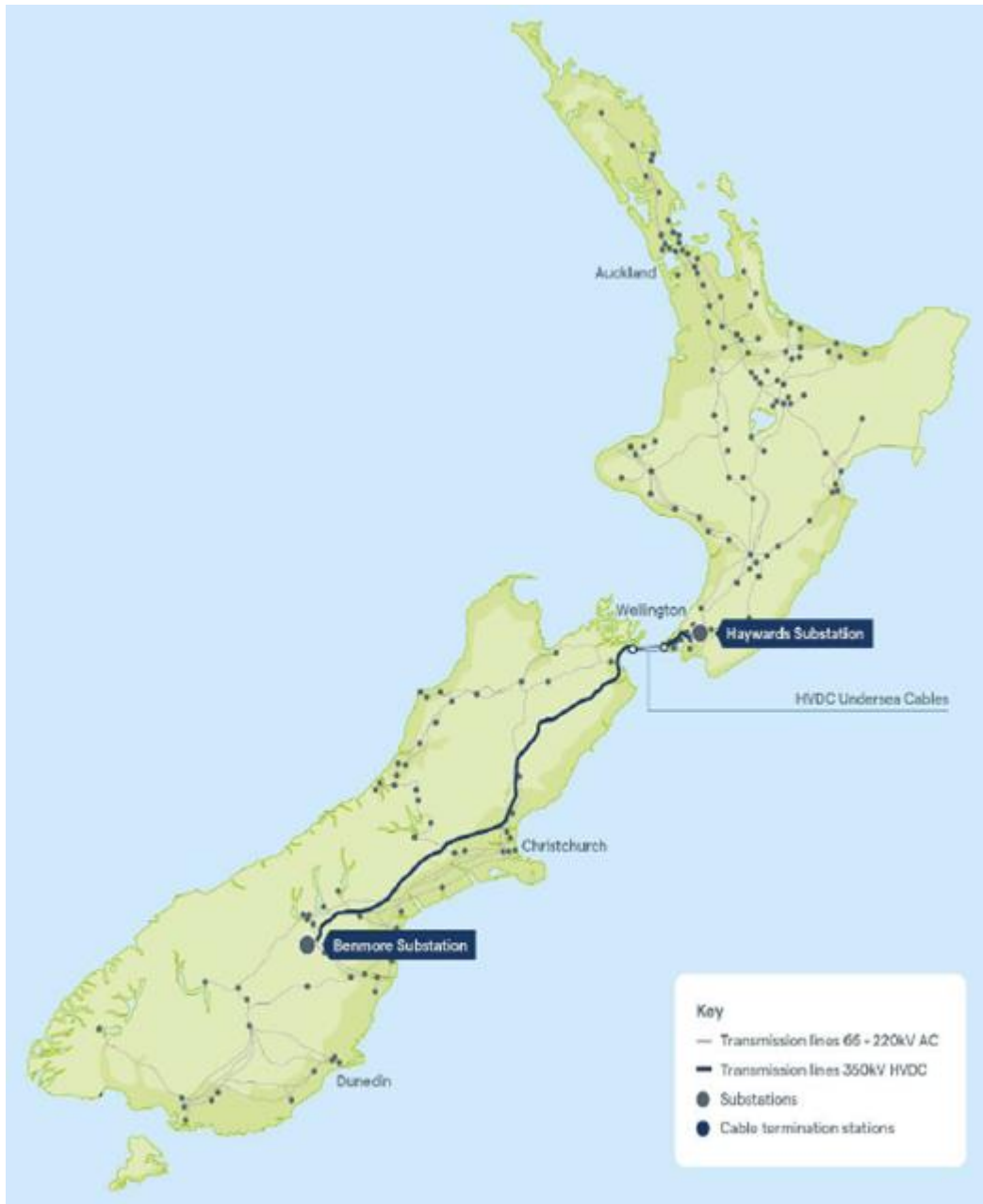
Figure 2.1 Overview of the transmission network showing the HVDC link 34
